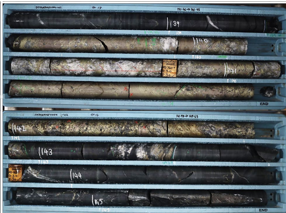
Figure 4: DD24KPMET004_W2 – 4.10m zone containing semi massive - massive sulphide and quartz-sulphide vein from 139.40m, comprised of ~35% pyrrhotite, ~30% pyrite, ~15% chalcopyrite, 20% quartz.
