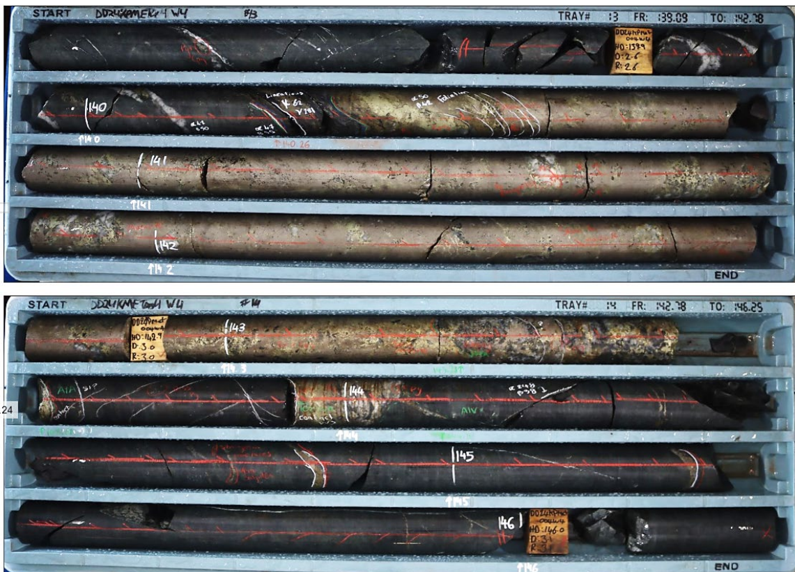
Figure 6: DD24KPMET004_W4 – 3.90m zone containing semi massive - massive sulphide and quartz-sulphide vein from 139.70m, comprised of ~45% pyrrhotite, ~35% pyrite, ~15% chalcopyrite, 5% quartz.
