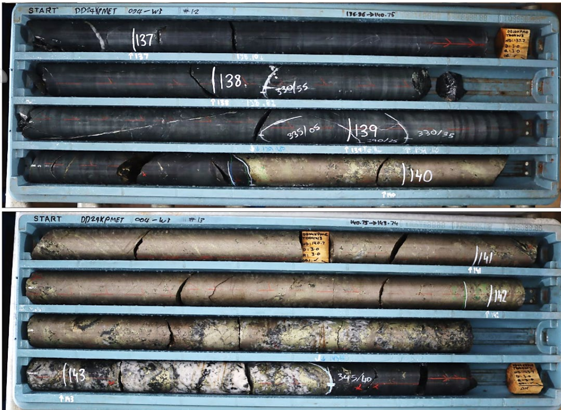
Figure 5: DD24KPMET004_W3 – 3.80m zone containing semi massive - massive sulphide and quartz-sulphide vein from 139.70m, comprised of ~35% pyrrhotite, ~35% pyrite, ~15% chalcopyrite, 15% quartz. Visible gold noted at 143.20m.
