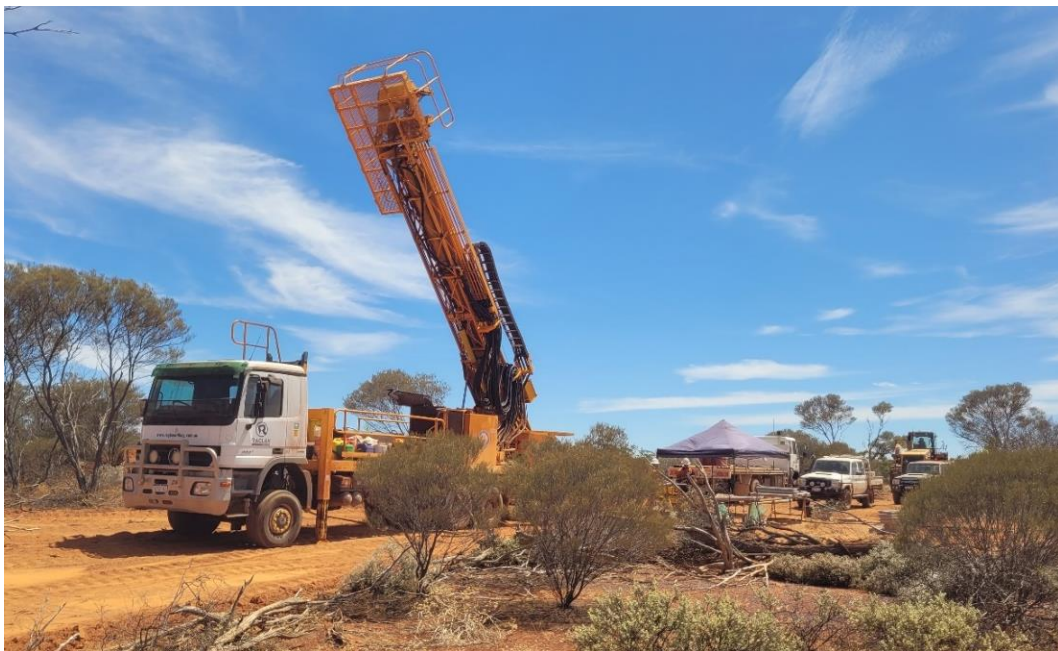
Figure 1: Line Hydrogen Pty Ltd contracted diamond drill rig drilling geotechnical hole for trial open pit as part of heap leach feasibility study
