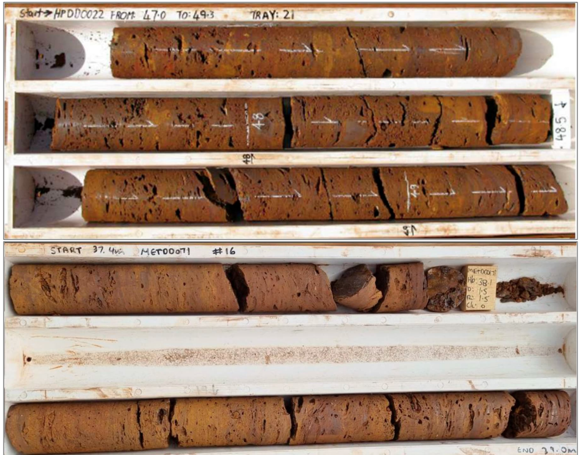
Figure 3.6: Diamond drill core photography of Dales Gorge Member hardcap ore type
