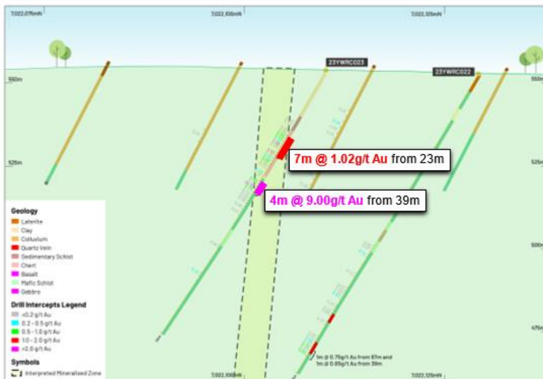
Figure 2: Cross section at Barwidgee Fault Prospect drilling.
