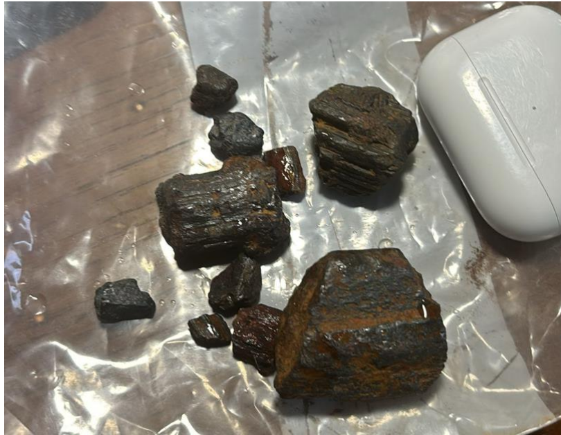
Figure 3: Coarse rutile nuggets from location MRGR0001 within the Minta Project. The nuggets were collected from a previous road base quarry. The nuggets are identified as coarse rutile and are estimated to contain 95% - 98% TiO_2 . See cautionary statement under Figure 2.
