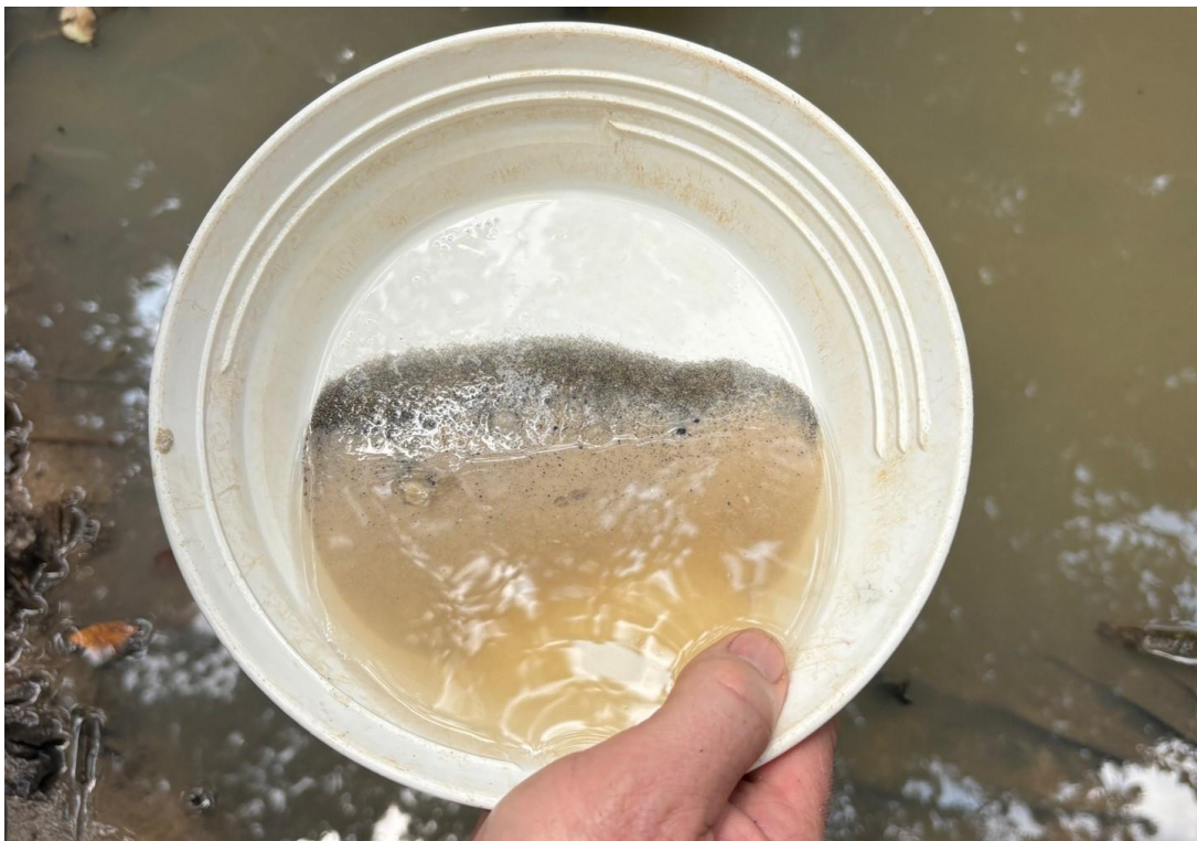
Figure 4: Rutile in a panned alluvial sand concentrate sample from Dormer hand auger. Sample was taken from MRAU0003 from surface and panned to a concentrate for mineral identification. Estimated in-situ rutile grade range within the sample of 1% -3%. See cautionary statement under Figure 2.
