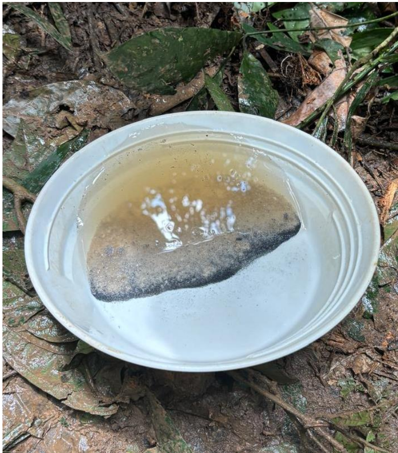
Figure 2: Rutile identified in a panned alluvial sand concentrate sample from Dormer rig. Sample was taken from MRAU0001 in metres 2 - 3 and panned to a concentrate for mineral identification. Estimated in-situ rutile grade range within the sample of 1% - 3%.
