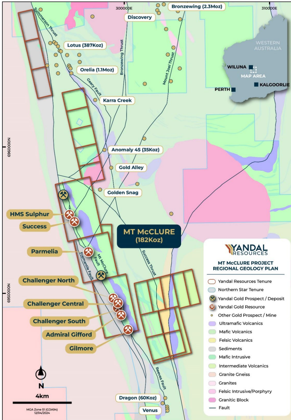
Figure 8: Mt McClure tenement plan showing the location of major prospects, interpreted bedrock lithology, major structures and proximity to nearby mines.
