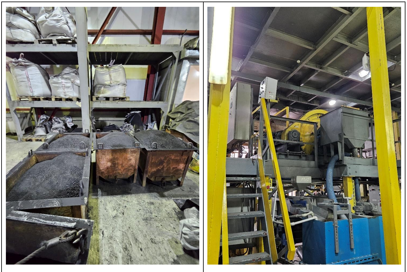
Figure 5 - Sarytogan Graphite after first stage crushing to 5mm size (LHS) and mill in Karaganda laboratory for next stage (RHS).
