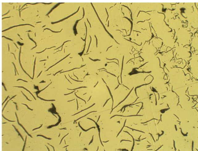
Figure 1 - Photo micrographs of grey cast-iron made with Sarytogan "Micro 80C" Graphite
