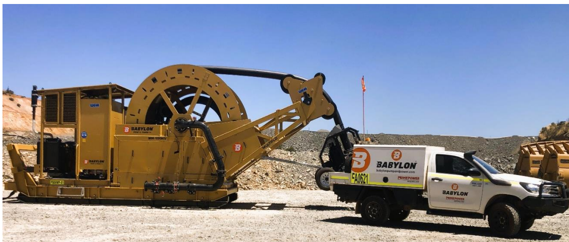
Highwall pump on site prior to commissioning at a major WA gold mine
