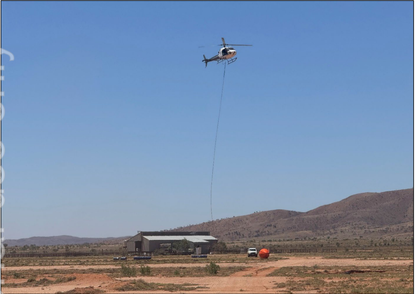
Figure 13: Airborne Magnetotelluric (MT) Survey over the Mundi Mundi Plains at the Broken Hill Project
