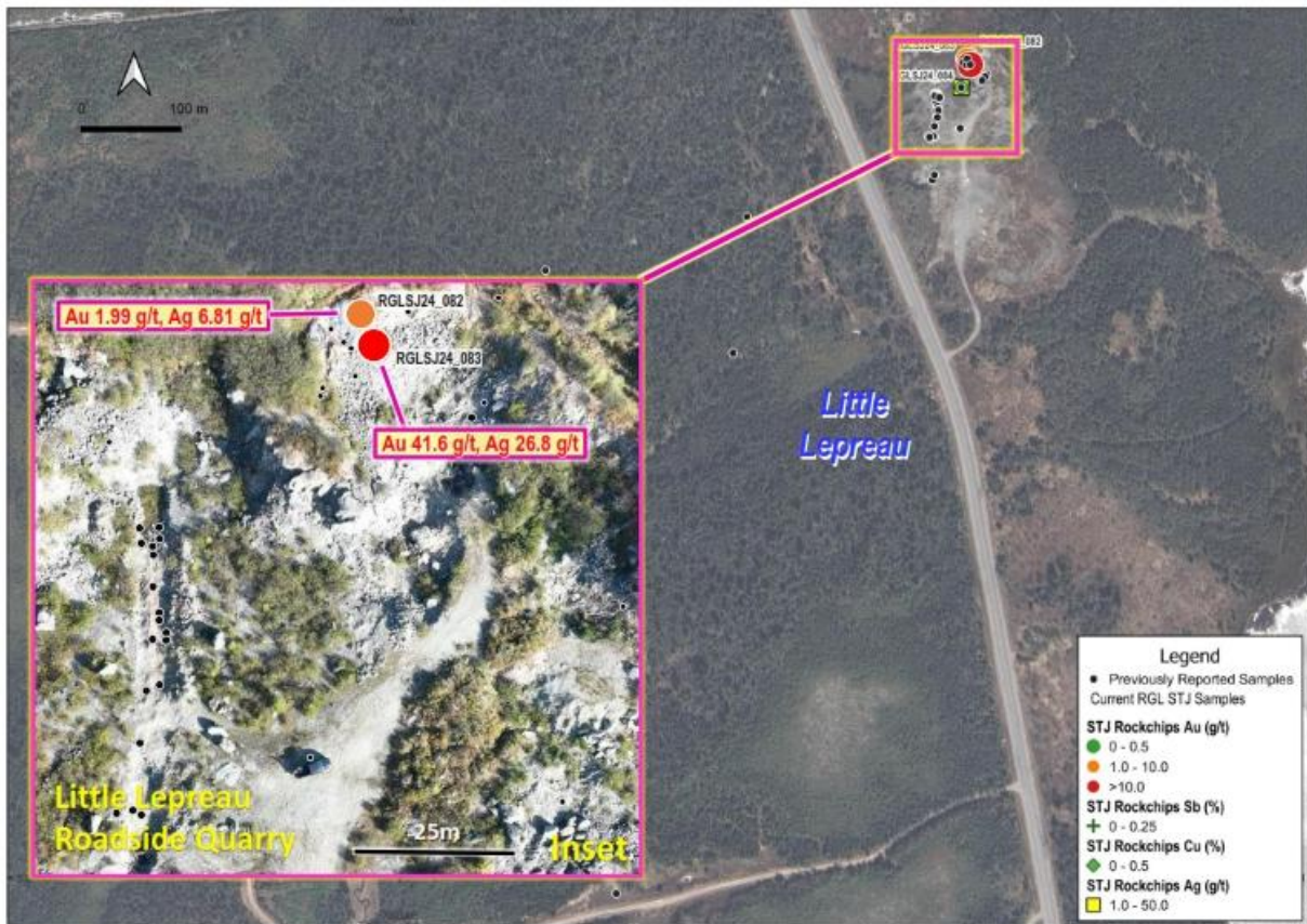
Figure 3: Little Lepreau prospect location showing previous rock chip sampling locations and highlighting significant multi-element results.
