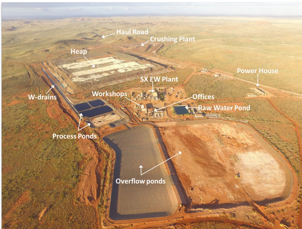
Figure 5: Whim Creek Site Plan showing the location of the Heap Leach Infrastructure
