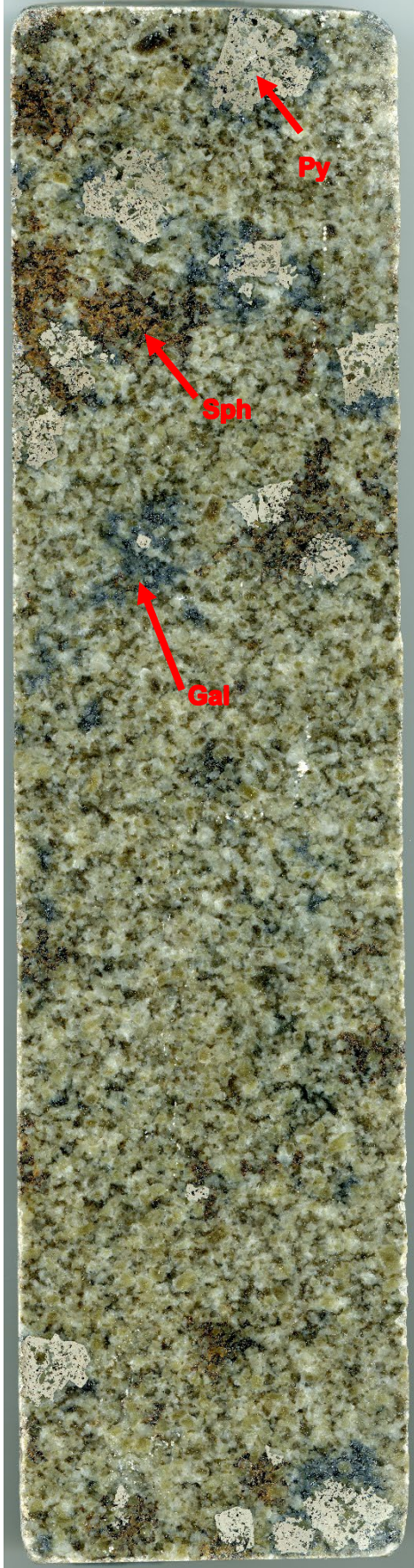
Figure 4: Polished half HQ core from MWDD002 340.25-340.45m displaying pyrite (Py), sphalerite (Sph), and galena (Gal) within a strongly sericite altered albitised leucogranite. This sample is part of a meter section (340-341m) that assayed 9.92g/t Au, 38.7g/t Ag, 0.45% Pb, 2% Zn.
