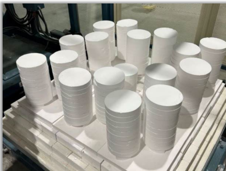
A production batch of densified, sintered HPA disc tablets (each tablet ~850g with density of >3.5g/cm 3 )
