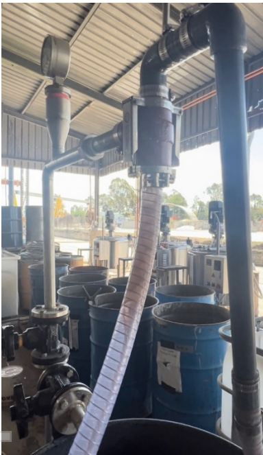
Figure 2a: Pilot plant cyclone rig in action treating material from the Lindfield Project
