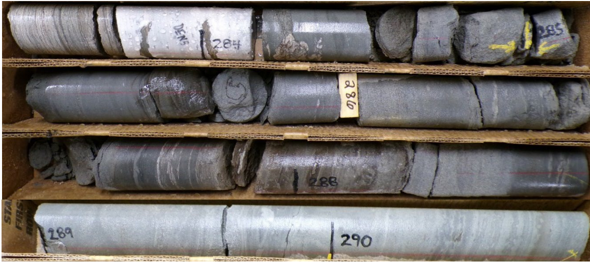
Figure 2. High-grade drill-core from 86.6-88.5m (285-290ft) in RMDD001 which assayed 3,070ppm Li
