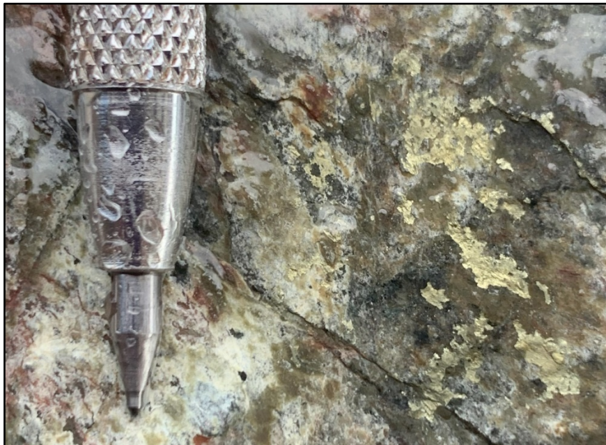
Figure 14. Trace chalcopyrite (copper mineral) on joint surface at 427.3m
