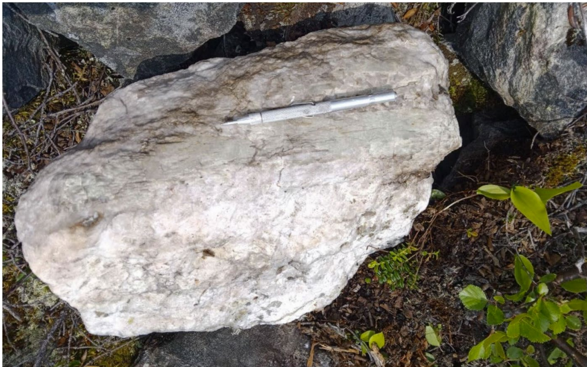
Figure 6: One of the spodumene-bearing pegmatite boulders found at Petit-Léran. Several of these boulders were found in an area with a 50m radius up-ice of the 2023 discovery.
