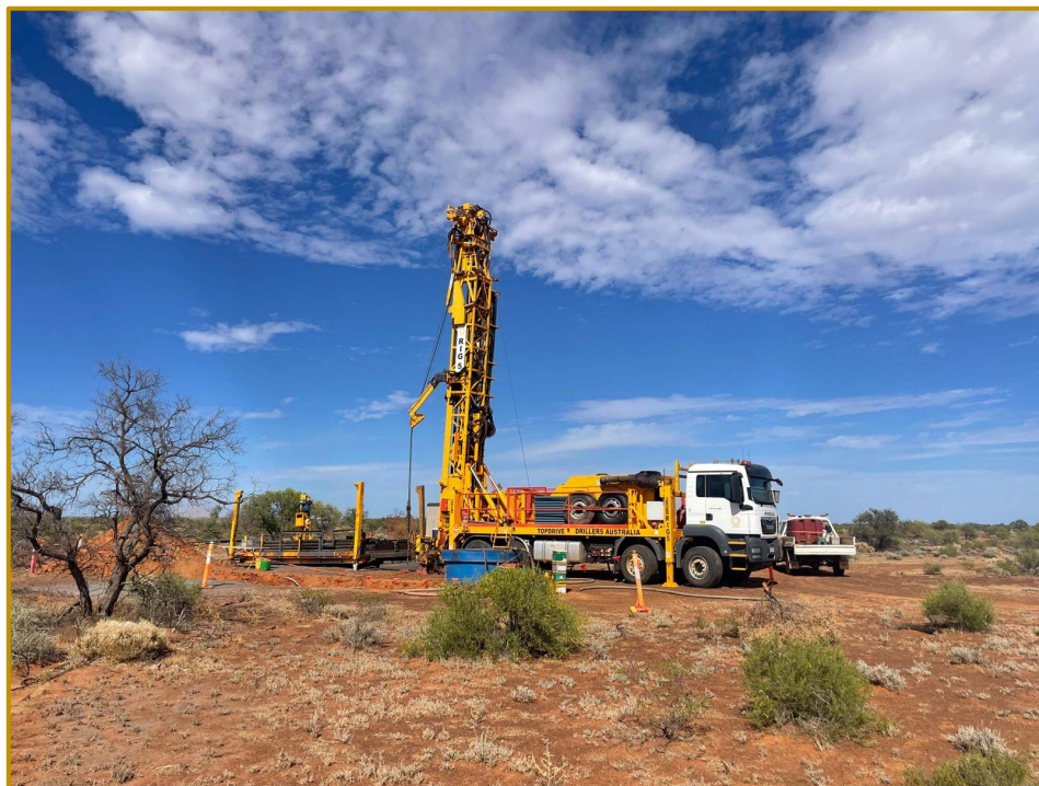
Figure 8. Core drilling at the Byro Project.
