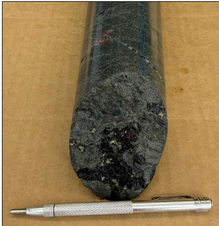
Photo 2. Chalcopyrite in a vuggy quartz vein at 170.4m in SJD001.
