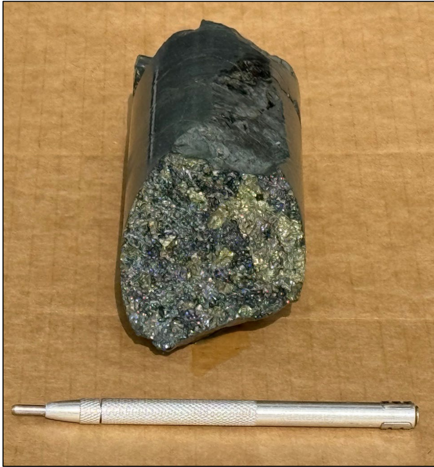
Photo 1. Chalcopyrite, chalcocite and minor pyrite in vuggy quartz vein at 160.7m in SJD001.
