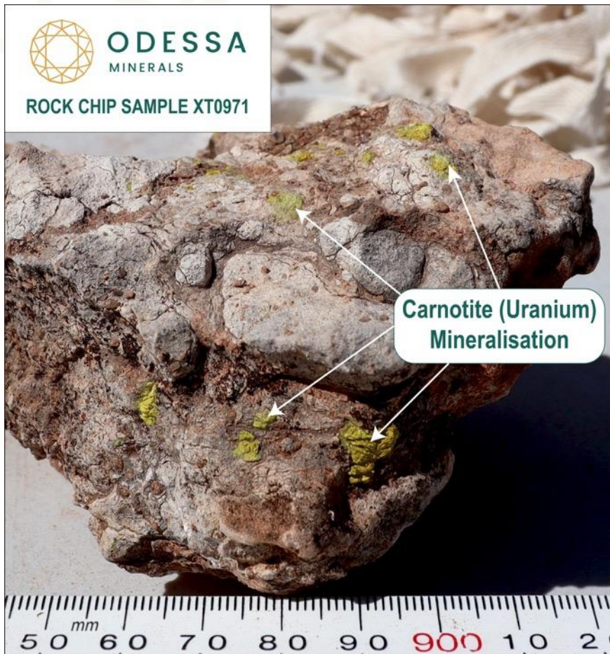
Figure 5: Carnotite (uranium) mineralisation within reworked siliceous calcrete at Baltic Bore in sample XT0971.
