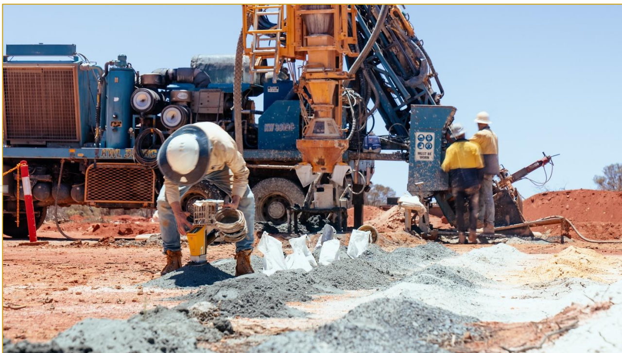
FIGURE 13: GEOLOGIST DAVID MAZUREK SCANNING RC SAMPLES WITH A HANDHELD XRF DEVICE AT MULGA BILL. IMAGE CREDIT: INSPIREAL FILMS
