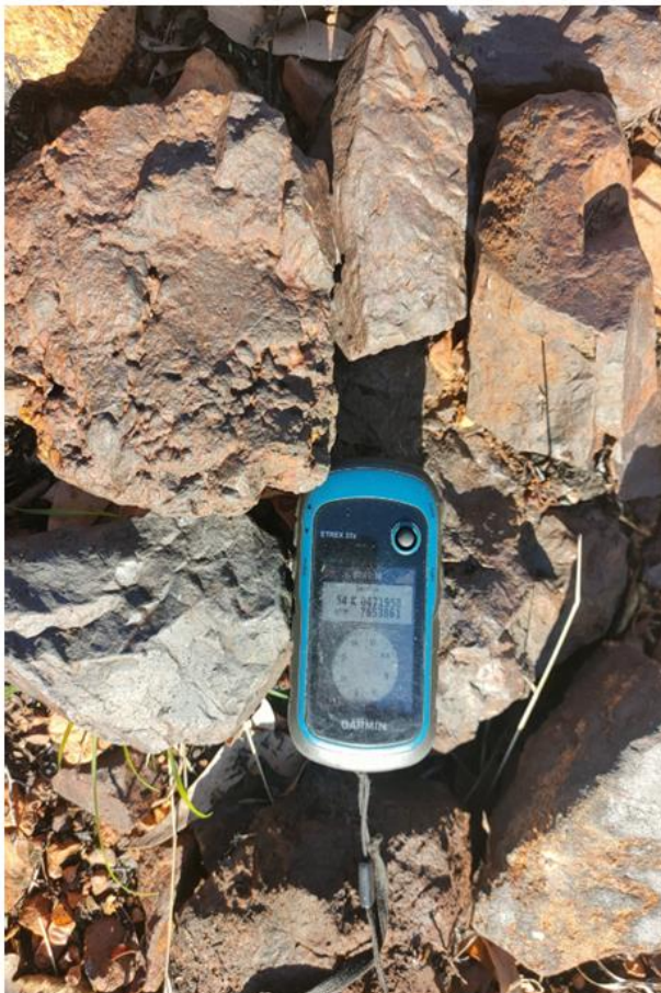
Figure 8 – Fe rich rock with Cu anomalous content at 7653861 N / 0471950 E
