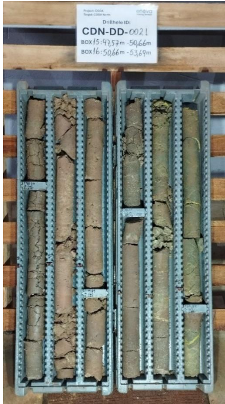
Figure 6: Diamond drill core within saprolite and saprock representing kamafugite litho-unit
