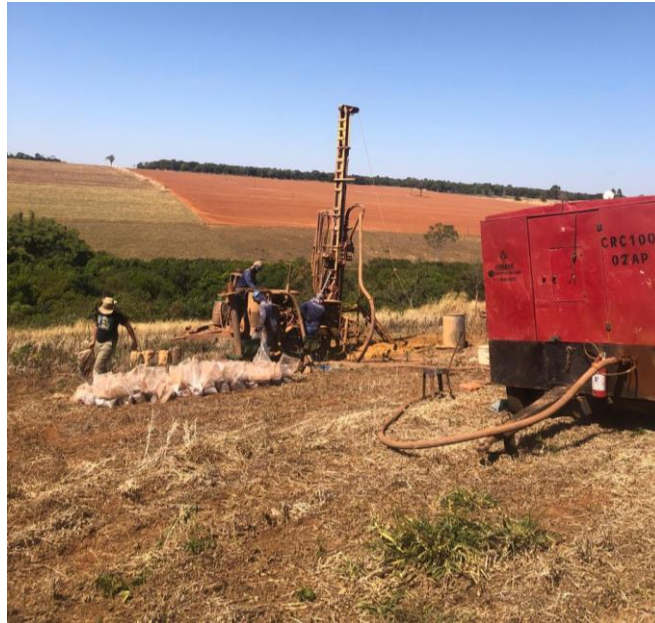
Figure 4: RC drilling rig in CODA North Project site operating in our REE mineralisation area (Sample bags are arranged in an array prior to logging)
