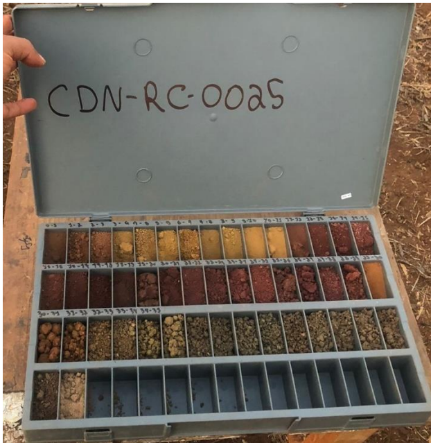
Figure 10: RC drill chips of variegated colour of saprolite are stored in chip library
