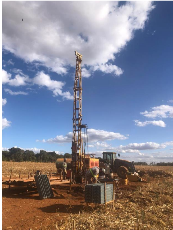
Figure 7: Enova's diamond core samples are being stored in the diamond core box
