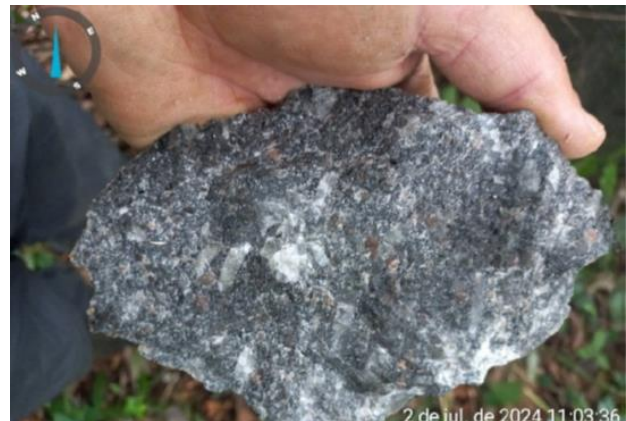
Figure 15: Coarse-grained nepheline syenite with a coarse equi-granular texture formed by the intergrowth of feldspar, nepheline, and mafic minerals
