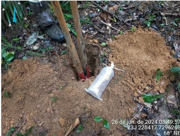
Figure 12: Pit sampling from sub-surface layers by contract geologist's team in July 2024
