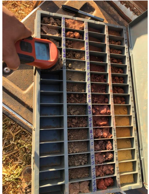
Figure 9: Enova's professional geologist is checking the magnetic susceptibility of saprolite drill cuttings during logging
