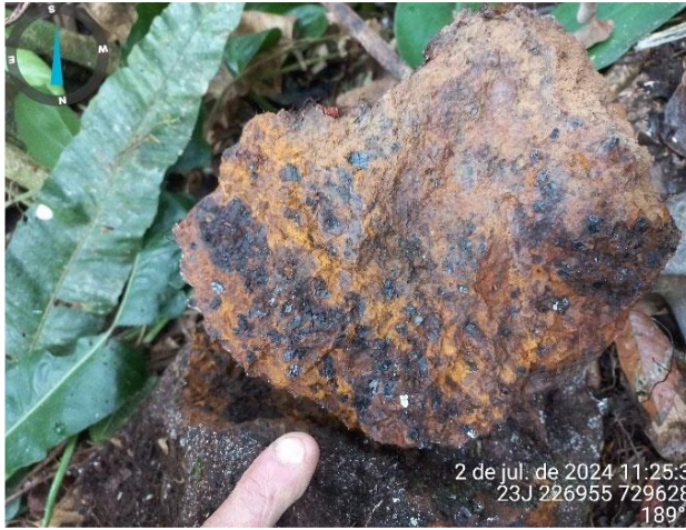
Figure 16: Segregated magnetite-rich layers alternating with heavily altered ferromagnesian minerals, likely of olivine origin (JUQ-RO-0022)
