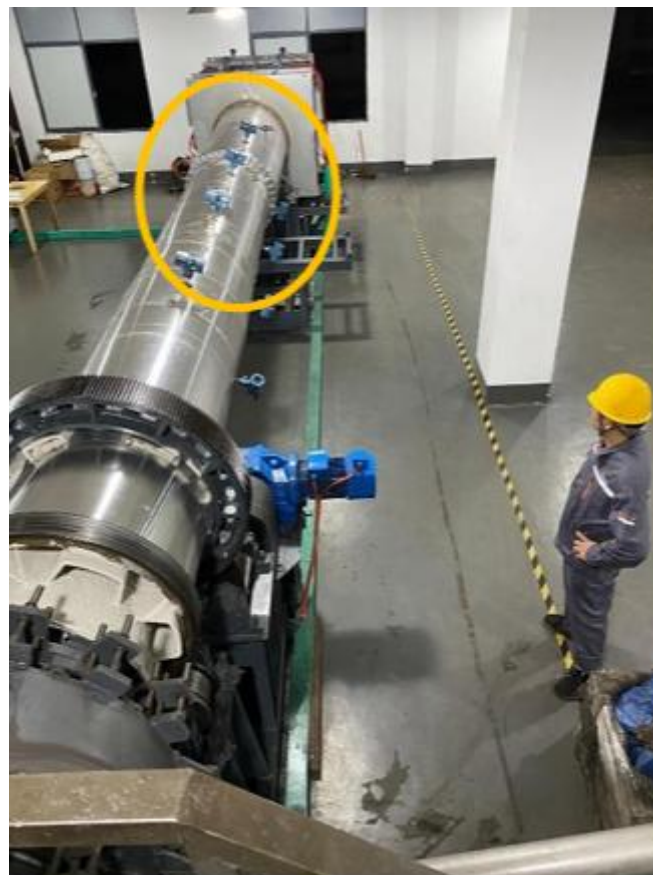
Image 4: Calcining Kiln with temperature gauges highlighted
