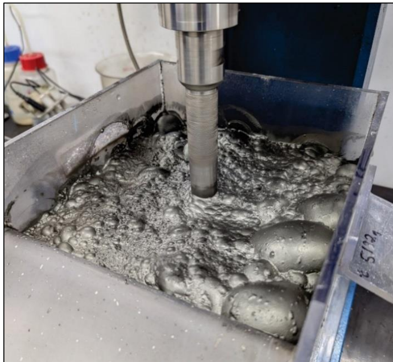
Figure 1: Copper-antimony-silver concentrate from Bulla Park, first flotation test run, at Core Resources Pty Ltd
