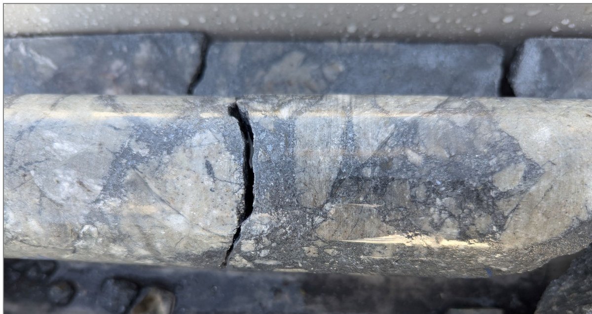
Figure 6: Core photo of the high-grade Sb interval in RDRC067 highlighting brecciated ultramafic at 239.4m. Refer ASX Release 26 August for full context)
