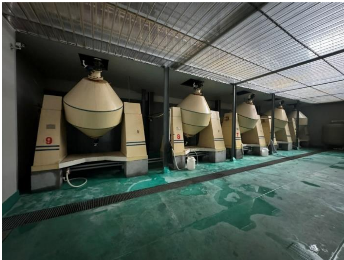
Figure 2: Left: Acid leach in newly commissioned HPQ factory visited in Lianyungang
