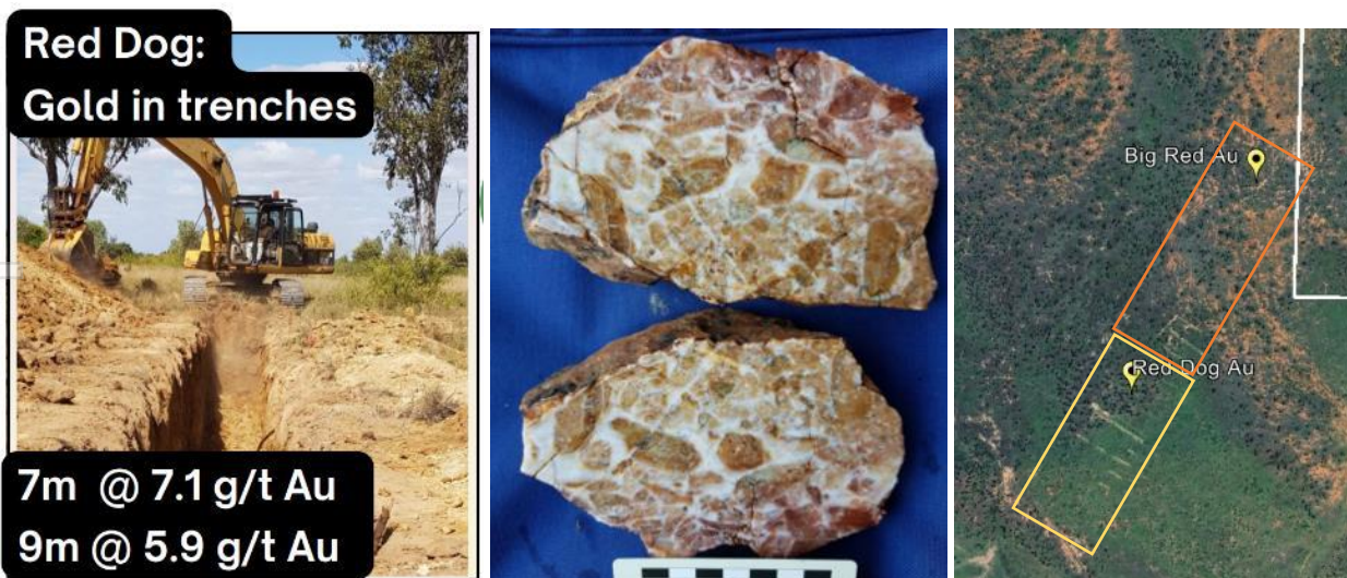
Figure 2: Big Red (Red Dog) Project –Past trenches; quartz breccias; area of past trenches (yellow rectangle) and planned extensions (orange rectangle)
