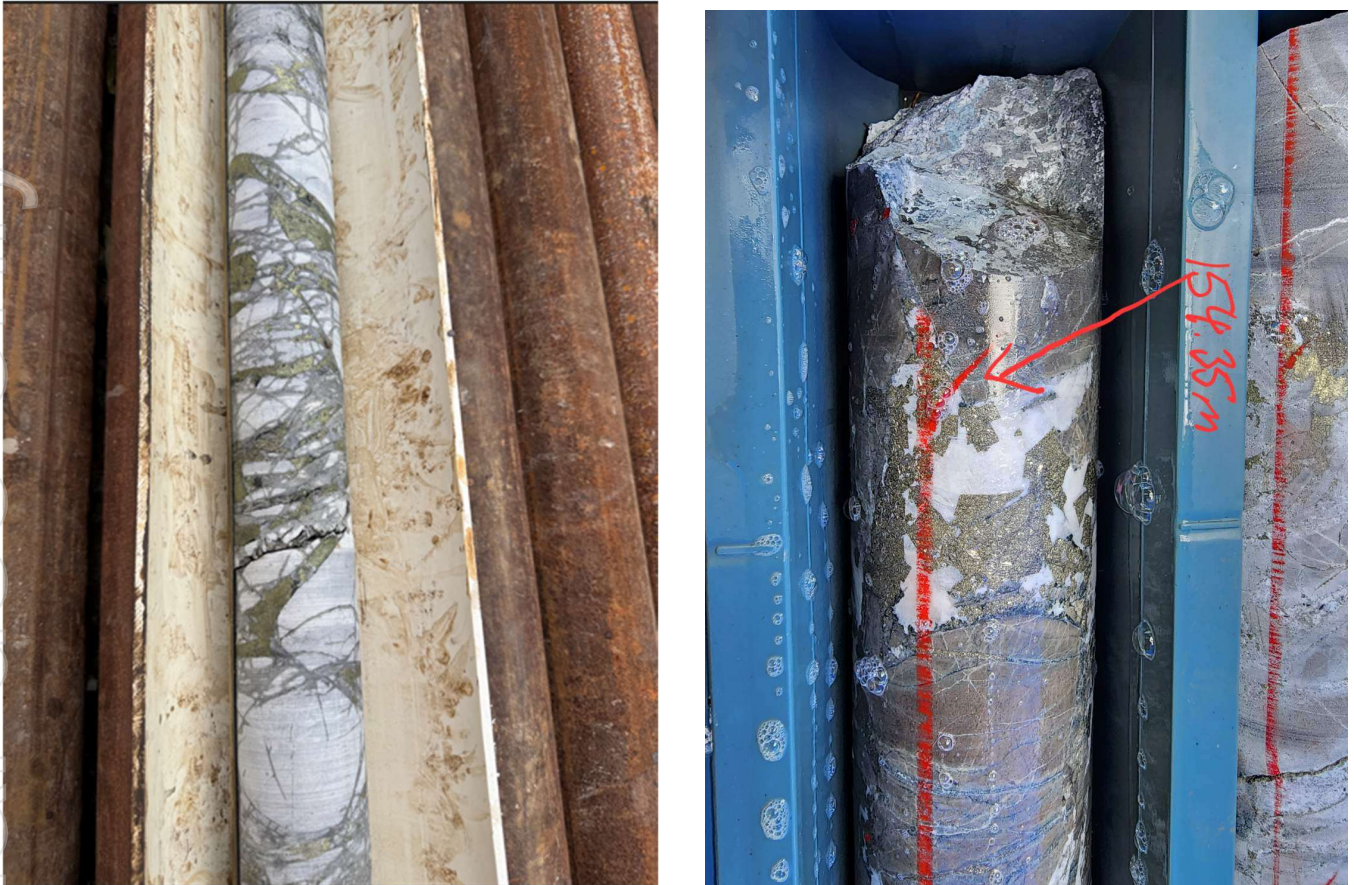
Figure 2. Chalcopyrite/Pyrite infill breccia examples from hole 24
