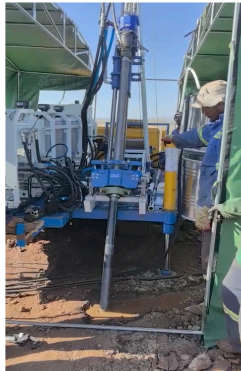
Image: Company owned diamond drilling rig commences drilling the first diamond drill hole at the Kameelburg Project.
