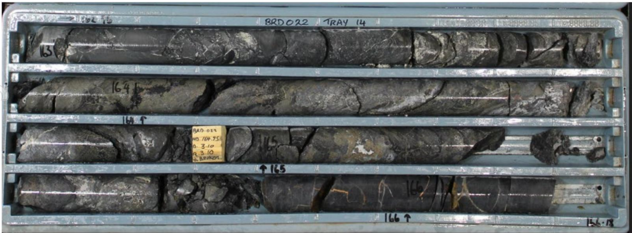
Figure 12: BRD022 main mineralised intersection between 163.6-166m down-hole. Intercepts included 2.4m @ 0.6g/t Au, 5g/t Ag, 1.9% Pb and 3.7% Zn including 0.5m @ 1.47g/t Au, 3.6g/t Ag, 1% Pb and 0.7% Zn from 164.5m.
