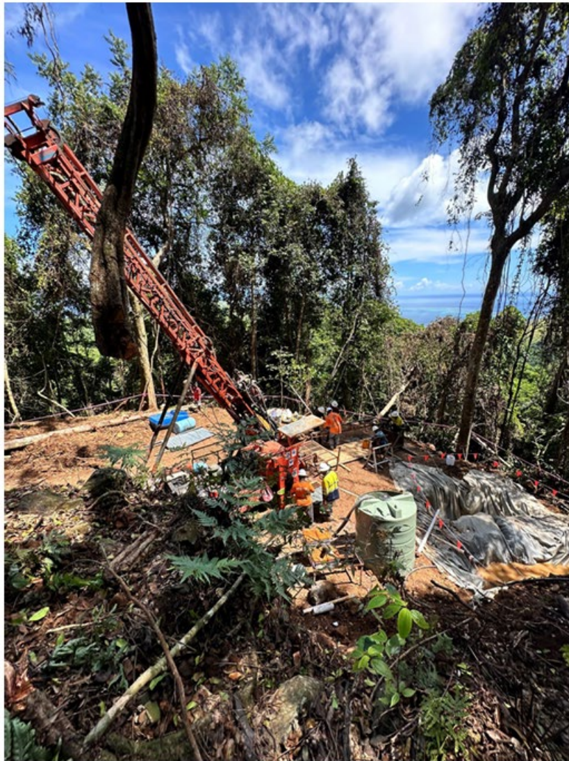
Figure 4 – Diamond drilling at Viani
