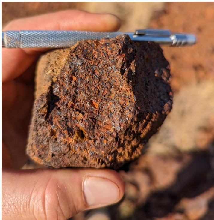
Figure 17: Robe River pisolite hand sample located from Mesa 3 (200m west of tenement boundary) showing representative Robe River pisolite found on Mesa 1 and Mesa 2
