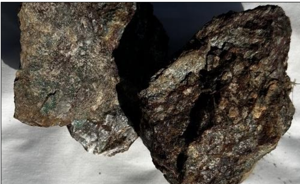
Figure 13: Lone Star Prospect sample TEM15 that assayed 4.11% Cu and 82.2 - 101 g/t Au (101 g/t Au = 3.2 Oz/t Au) 10
