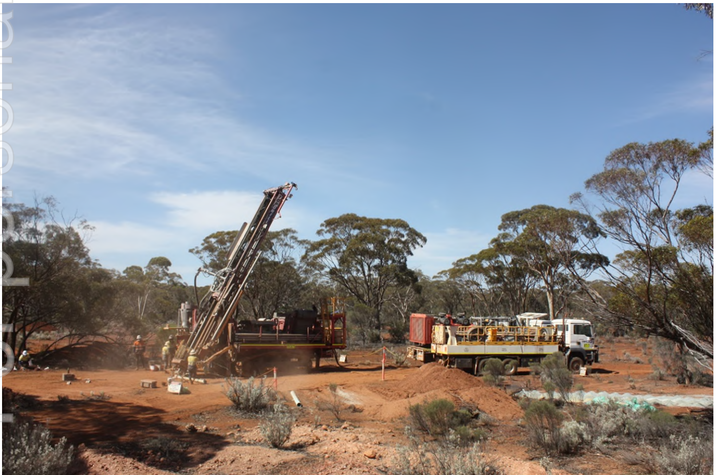
Figure 1: Topdrill RC rig drilling at the Ada Ann Prospect, Bonnie Vale Project
