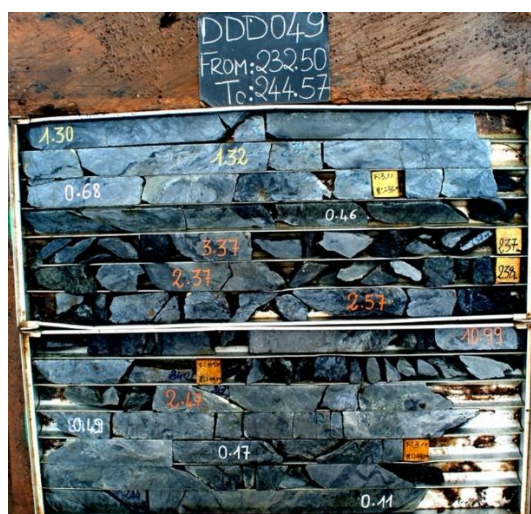
Figure 6: Photographs of the intersection of 65m at 5.6 g/t of gold from 177m of the diamond drill core from drill hole DDD049.
