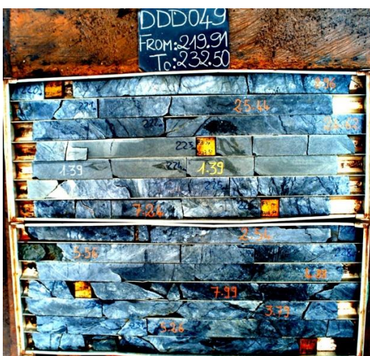
Figure 6: Photographs of the intersection of 65m at 5.6 g/t of gold from 177m of the diamond drill core from drill hole DDD049.
