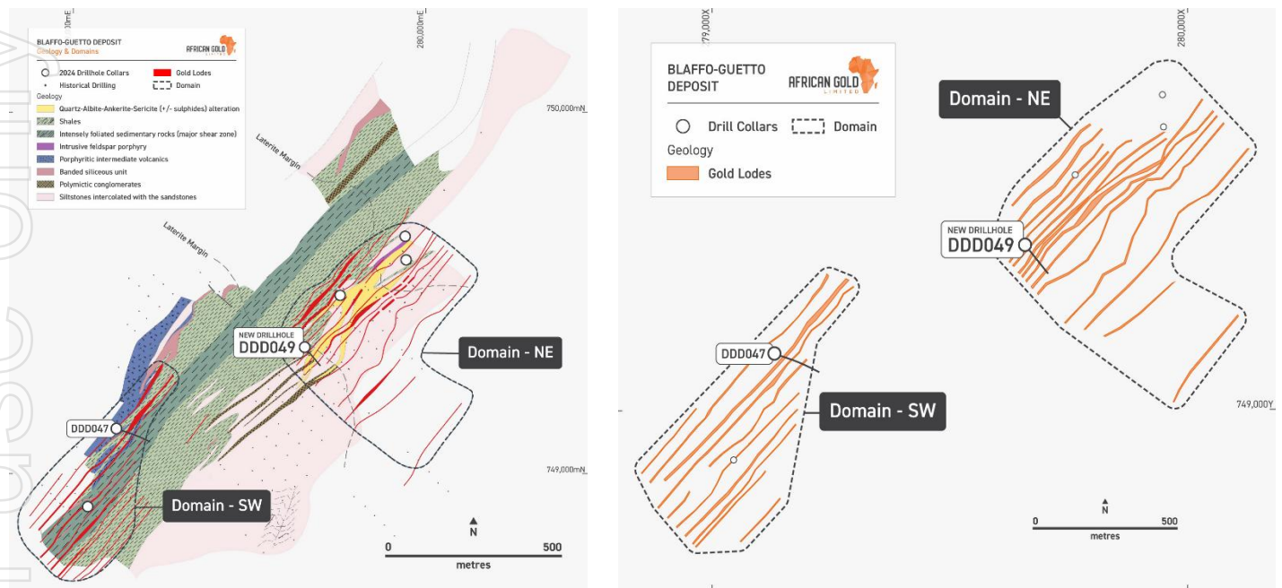
Figure 7: (left) Geological map of the Blaffo Guetto prospect showing location of the new drillholes (the collars are shown as the dots); (right) gold lodes and trace of the DDD049 drillhole. Trace of the DDD049 is shown for reference.
