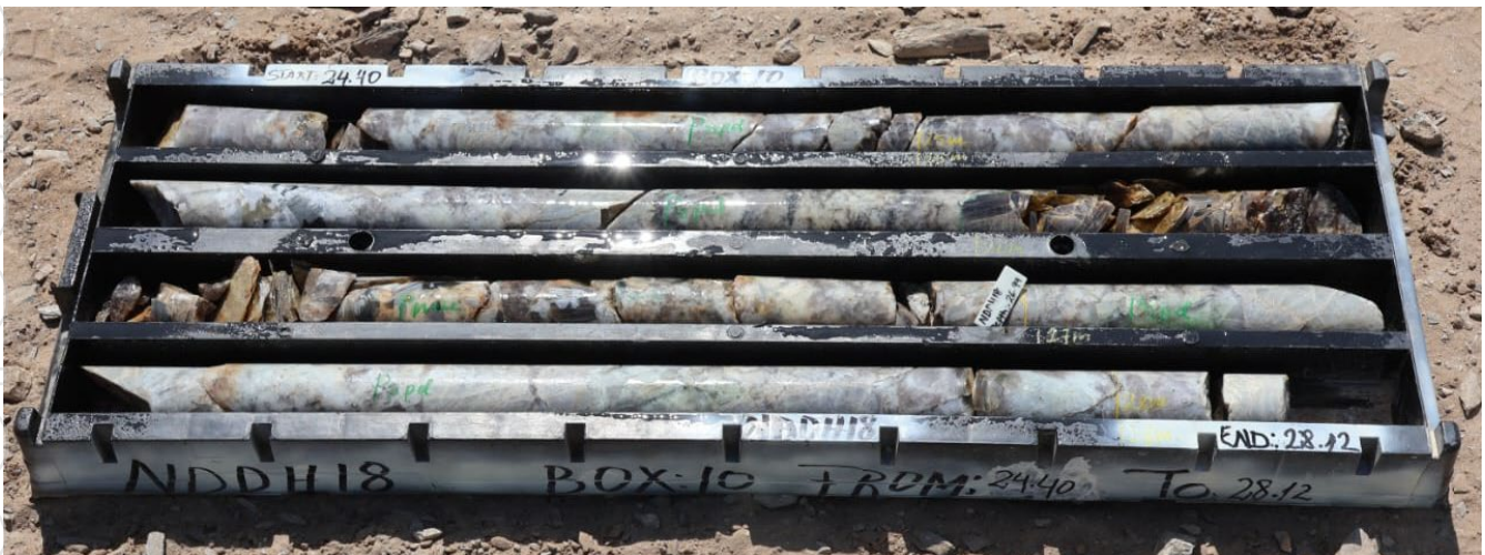
Photograph 2: Core from hole NDDH018, Interval 24.40 to 28.12m. Spodumene mineralisation from the start of the tray until 26.00m and then from 26.72m to the end of the tray assayed >2.00% Li 2 O.
