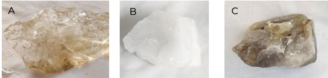
Figure 4: Kingsgate quartz samples (A) translucent (KQA-001), (B) white opaque (KQA-009) and smokey quartz (KQA-011). Note these samples have been cleaned of superficial organic material and dirt using a diluted weak HCL solution and water.
