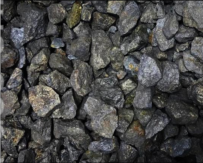
Photo 1. Mined and coarsely crushed Montezuma mineralisation. Representative sample assays of mineralisation only batches averaged 9.02% antimony (Sb), 769 g/t silver (Ag) and 15.47% lead (Pb)
