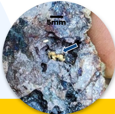
Visible gold in spoil 70m uphill from A1 – 429g/t Au (sample R0357)
