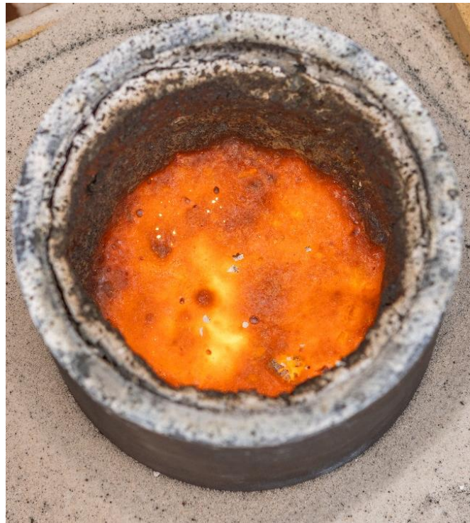
Figure 4: Conversion vessel with ferroniobium cooling following the test
