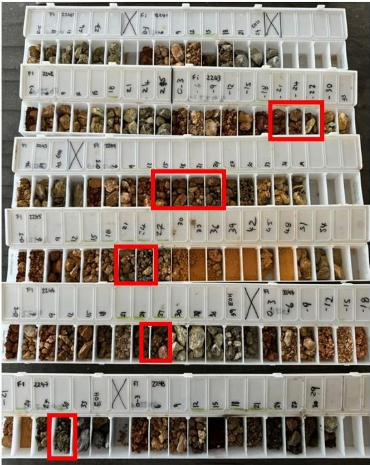
Figure 6: Currajong Prospect chip trays showing anomalous scandium (+100ppm Sc) intervals. Note each interval represents 3 metres downhole.
