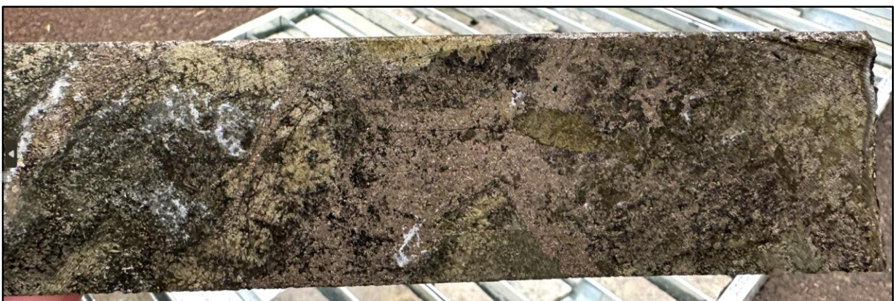
Figure 1. Core photo showing semi-massive pyrrhotite from 523.9m in ZRSD24174 at Gradina – 17.6g/t Au.
