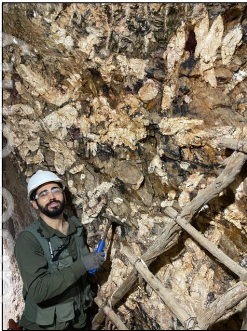
Figure 4a (left): Spodumene rich portion of the zoned pegmatite discovered at the Esperança project. Figure 4b (right): Large elongate spodumene crystals (Spd) up to 50cm in length showing homogeneous growth patterns amongst a quartz (Qtz) and Feldspar (Fdsp) rich matrix
