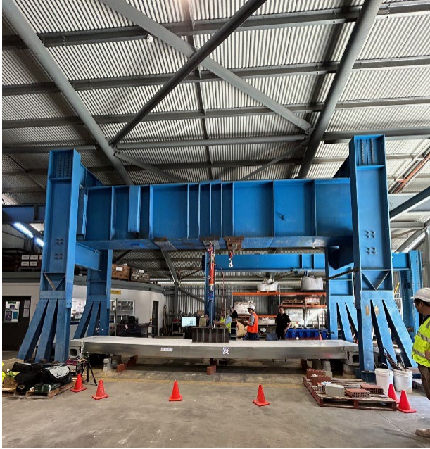
Above: Curtin University MDSB® Load Testing with SlimDek210®
