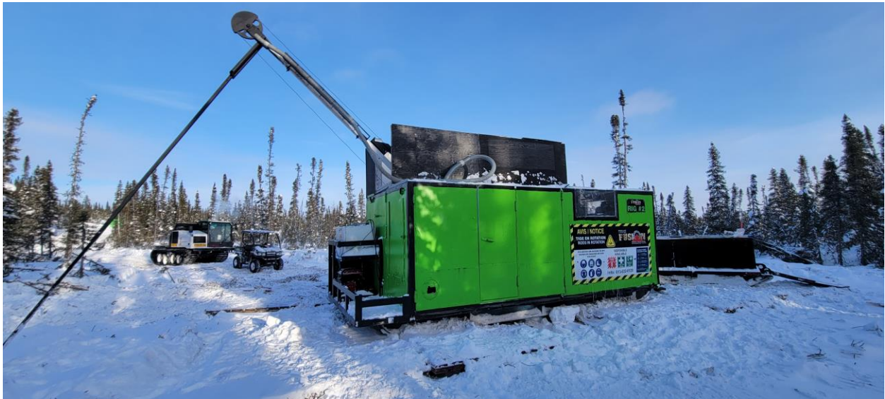
Figure 4: Drill rig on pad and ready to commence coring.
