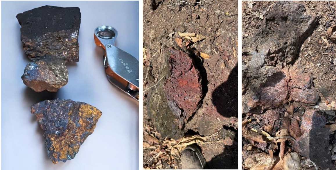
Figure 4: Gossanus sample and ferricrete out crop from recent field inspection
