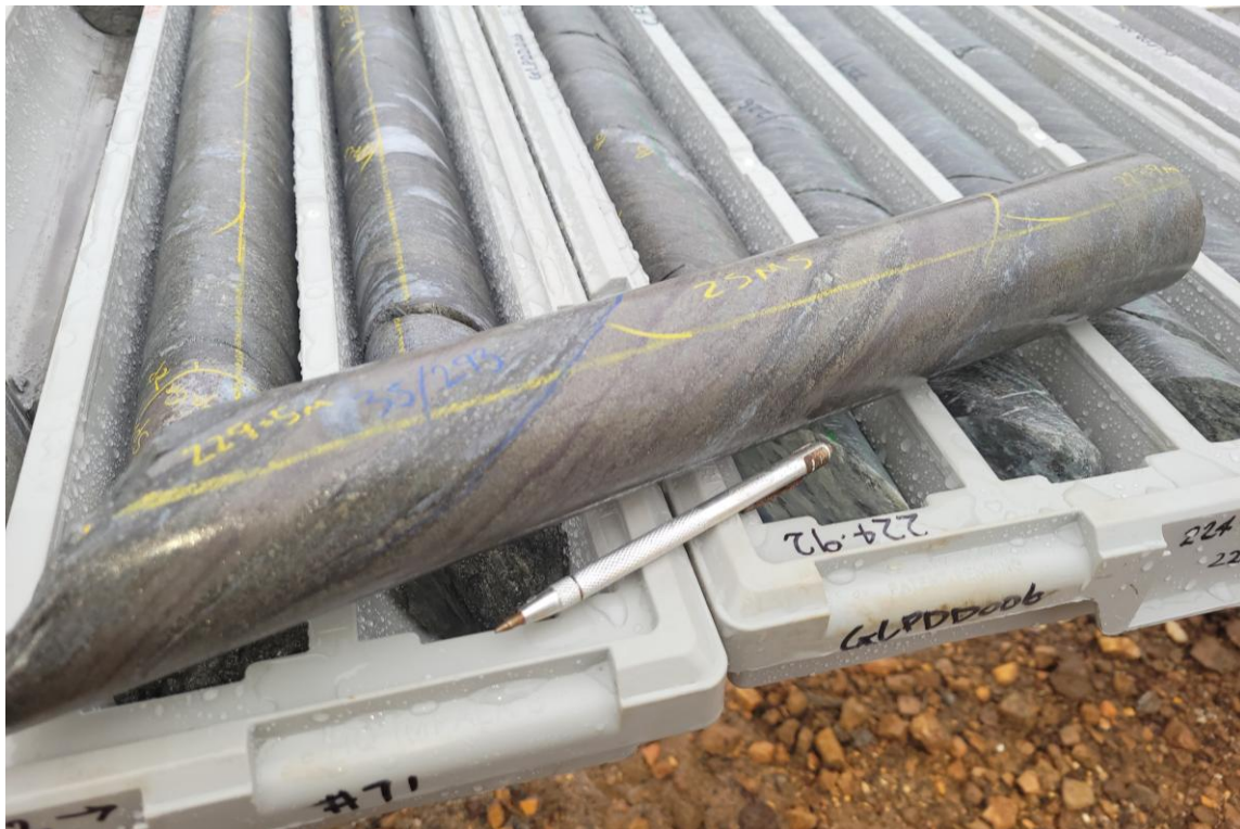
Figure 5: Photo of diamond drill core from GLPDD006 showing massive to semi-massive sulphides with banded pyrite (yellow) and sphalerite (red) with galena and chalcopyrite. This interval returned in sample GRD10725 (228.95-229.95m) 10.85g/t Au + 18.67% combined Lead-Zinc.
