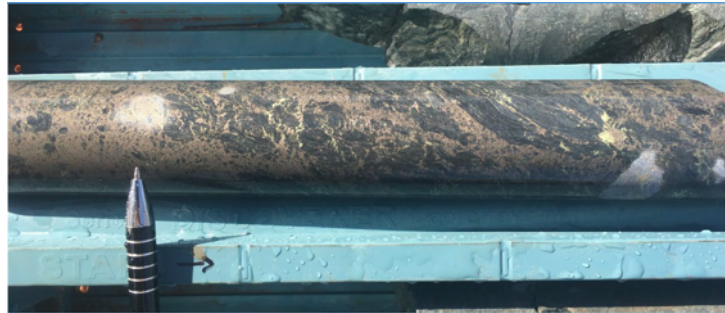
Figure 4 Wilga Downs Prospect - diamond core from hole 20WD001 at 552m depth showing semi-massive pyrrhotite (bronze colour) and chalcopyrite (yellow) CuFeS_2 mineralisation. Grade 1m @ 0.7% Cu and 0.7 g/t Au.
