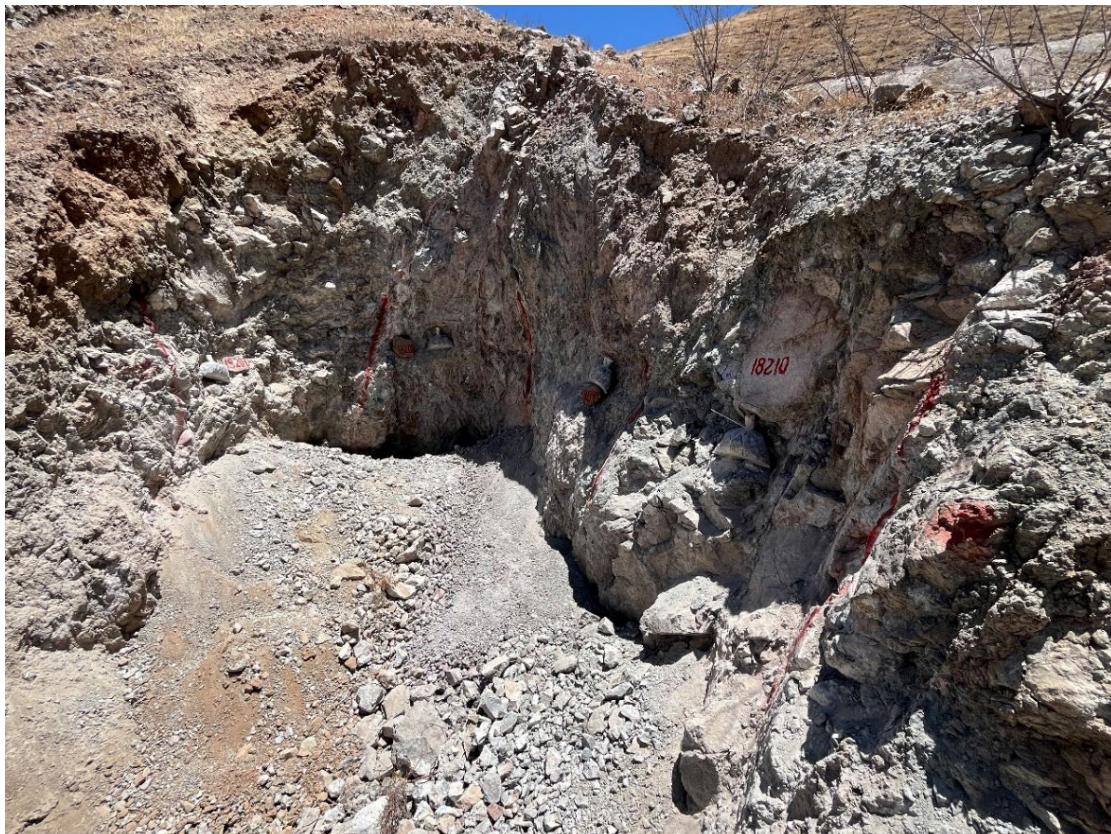
Figure 5: Channel 4 (viewed from north) sampled across brecciated and altered andesitic tuff outcrop exposed by old workings. Width of photo field of view is approximately 7m. Assay results returned over 0.00-5.50m (4.50m linear) are Au 0.011 ppm, Ag 3 ppm, Cu 1.03%, Mo 1 ppm, Pb 128 ppm, Zn 212 ppm.
