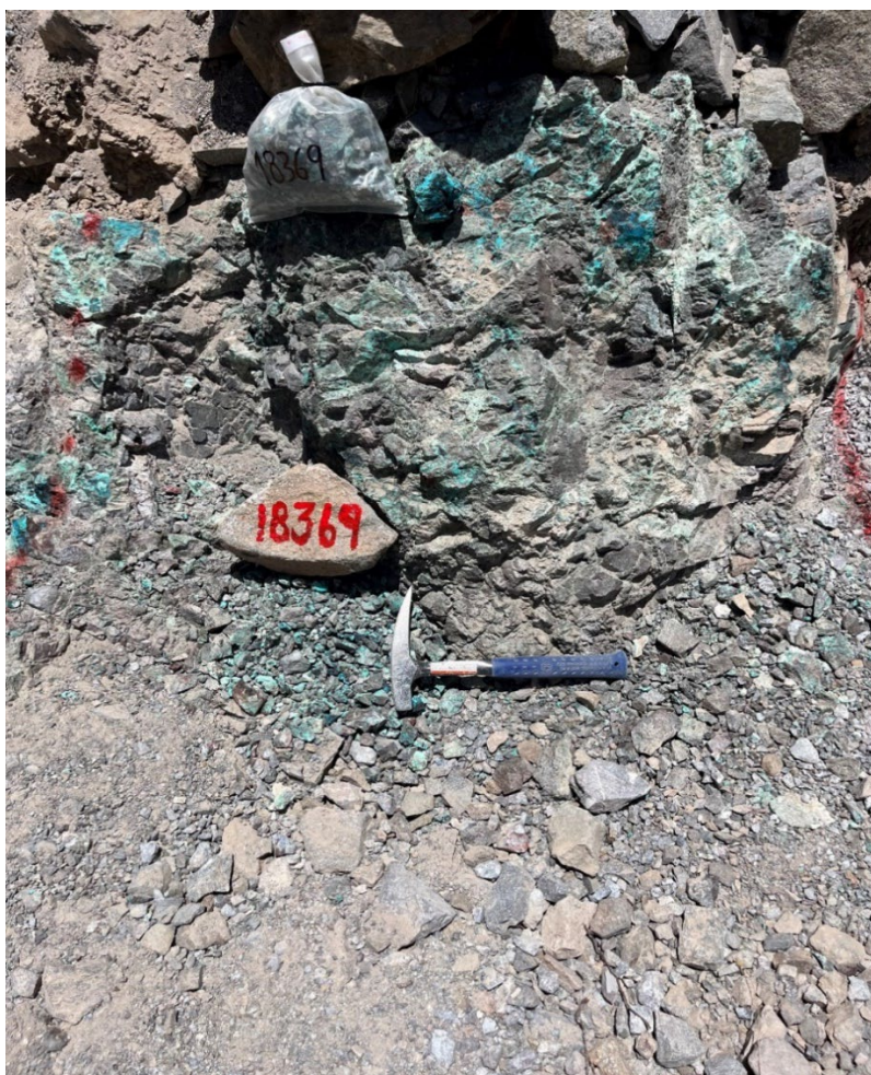
Figure 2: Cinto Project Channel 7, sample 18369, taken across mineralisation in brecciated andesitic tuff exposed by gully erosion. Sample length 1.1m. Assay results: Au 0.535 g/t, Ag 25 g/t, Cu 8.7%, Mo 1 ppm, Pb 283 ppm, Zn 873 ppm.
