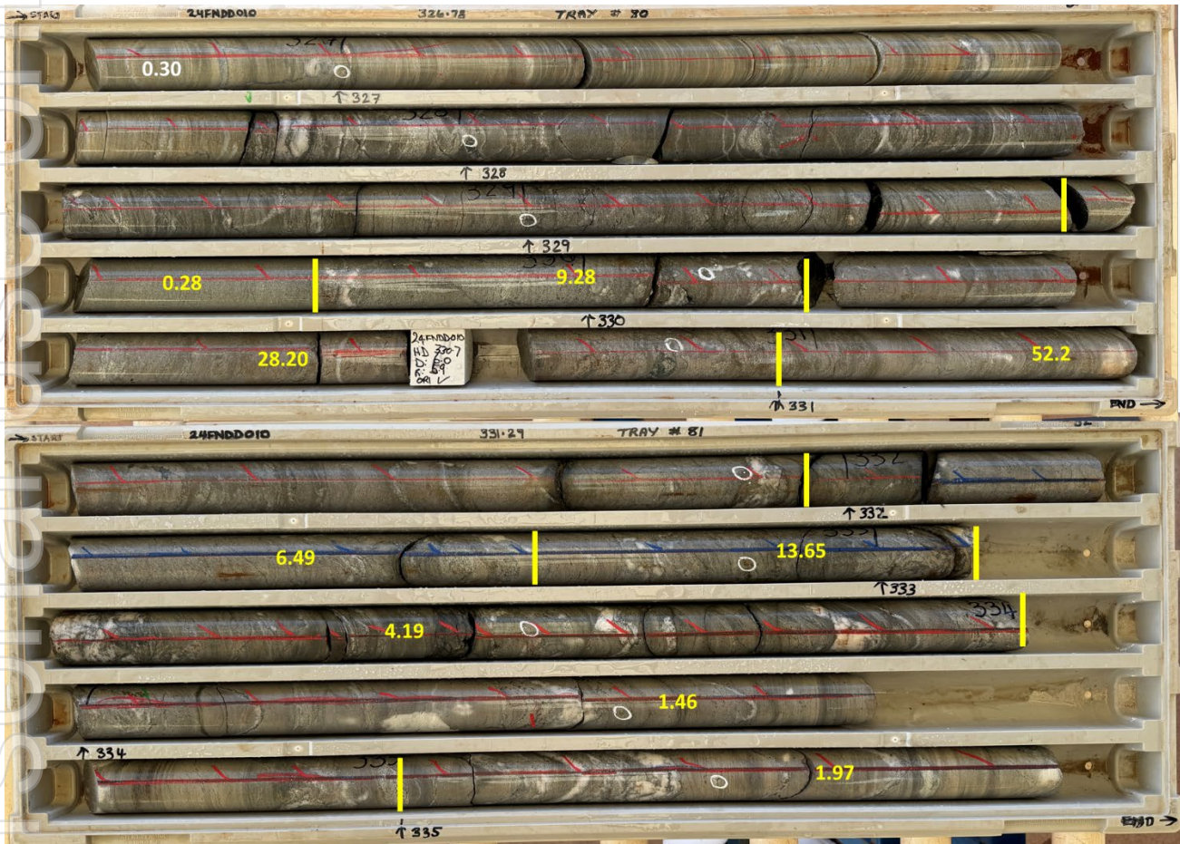
Plate 1 :24FNDD010 drill core from 326.78m to 335.6m with gold values (g/t) annotated in yellow
