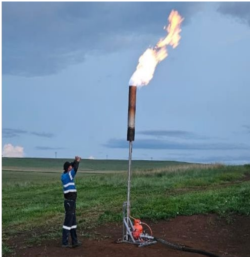
Figure 1: Gas flaring from well 271-06PT
